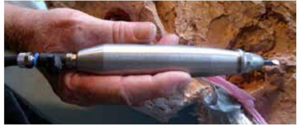
HW-90 Standard and extended length chisel shape needle holder and needle.
