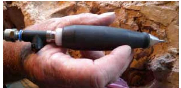
HW-70 Head with needle holder and needle. The 3 different diameters offered add to the range of work for micro (1.3 mm), medium (2mm) or heavy tips (3 mm).
