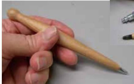
HW-1 Even running pneumatic air scribe with 3 springs of different hardness for various applications. It is good for beginning preparators. Choice of 2 mm diameter hard metal tungsten carbide tip or 1.3 mm diameter steel tips supplied with 5 extra tips. Hose and connectors included. Runs at 5.5 - 8 bar. (80 - 115 psi)
