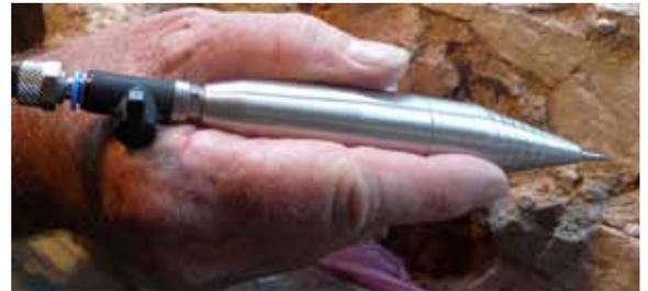
HW-70 The most versatile flying piston pneumatic air scribe because there are 3 different diameter heads and needles offered making it good for a wide range of work. It has a well balanced great feel. Hose, connectors and in line regulator included. Supplied with choice of 1.3 mm, 2 mm or 3 mm diameter standard length tip and associated head. Standard working length protrudes 10 mm from the head of the tool. Available in extended lengths by special order. Runs at .5-2.5 bar.
