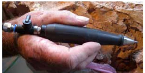
HW-90 This is the biggest and strongest for big jobs. It uses a 5 mm diameter chisel tip. It works great on hard matrix. Largest tool you can use in one hand allowing use in glove box. Comes with an inline regulator. Pressure should not exceed 4 bar (approximately 60 psi) to avoid damaging the tip.
