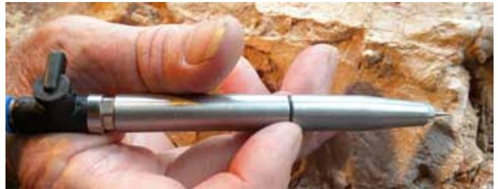
HW-1 - Needle holder and needle - Hard metal (2mm) or steel (1.3 mm) diameter
