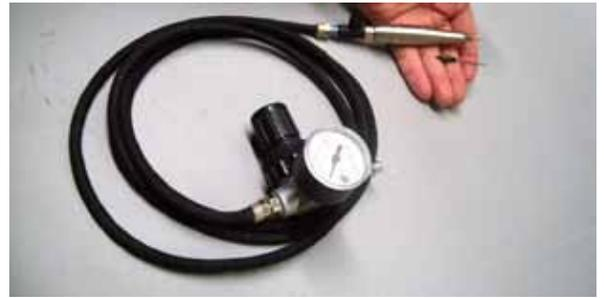
HW-80 The next most detailed flying piston pneumatic air scribe after the HW 322. Comes with 2 mm diameter head and needle. Hose, connectors and in line regulator included. Extended tip is advisable for hard to get areas. Operates at 0.5-2.3 bar (7-33 psi)
